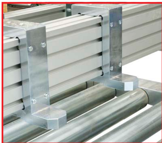
Facchini di prelievo pallets Pallets withdrawal devices
